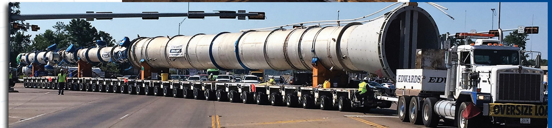
Barge roll-off of Gas Turbines weighing 650,849 lb. each.
